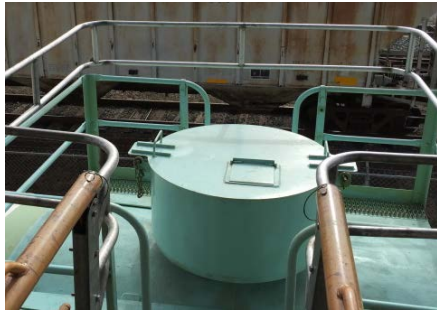
Image 3: Enclosed dome top fittings protection meeting AAR standard for new build
