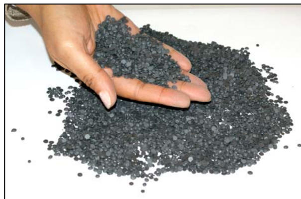
Figure 8: Shell sulphur-modified asphalt pellets.
